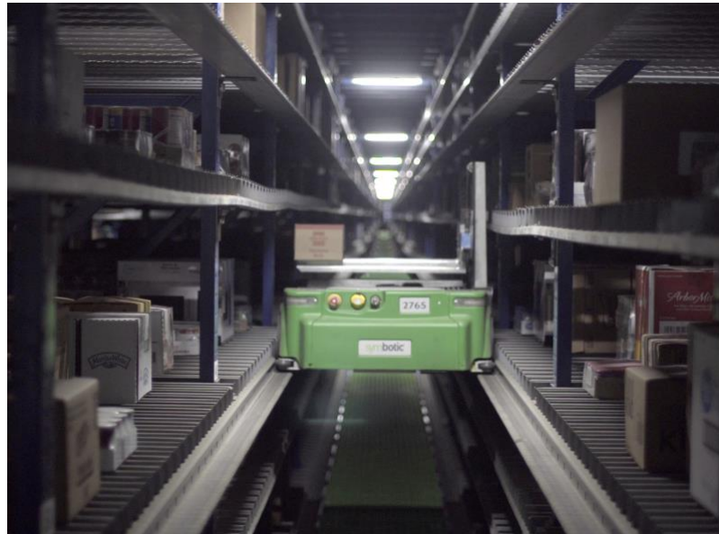
Figure 4. A Symbiotic Automated Storage and Retrieval System (ASRS) for Groceries
